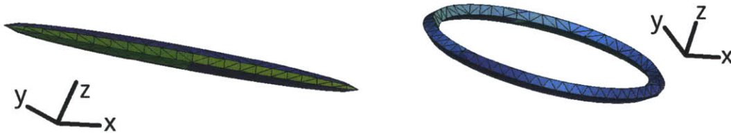
Figure 4-1: Example meshes of quasistatic structures considered, including a rod (left) of length 2400 nm & equatorial diameter 92 nm, and a torus (right) of major radius 36 nm and minor radius 2.5 nm
