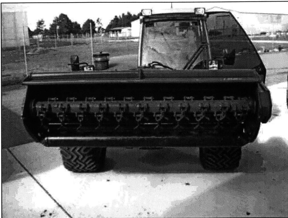
Figure 1: Image of a chain flail mower taken from http://scsc302.wikispaces.com/file/view/flail.jpg/187565895/flail.jpg
