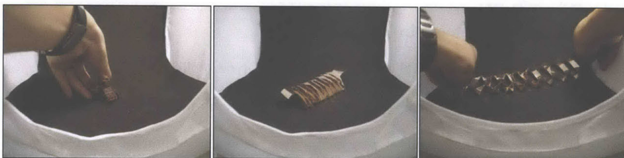
Figure 2.7b – Self-folding stretchable resistor after application of heat. The resistor can be compressed, as seen in the leftmost photo. The center photo shows the resistor in its neutral state, while the rightmost photo demonstrates the stretching capability of the resistor.
