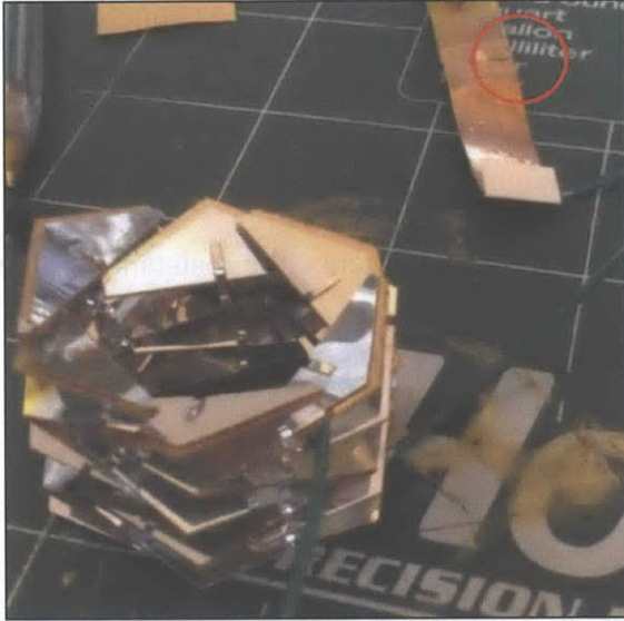
Figure 2.5a – Uncompressed switch – LED is off. Upper and lower tiles (which are connected to the circuit via the green wires) do not connect via conductive origami tiles.
