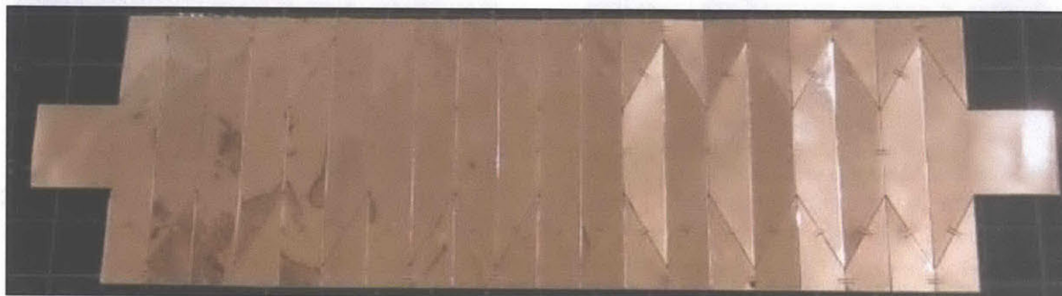
Figure 2.7a – Self-folding stretchable resistor before heating and self-folding.
