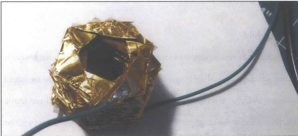
Figure 4.1 – A 24-winding hand-folded coil. The folded coil consists of copper material (to withstand high levels of current) insulated with Kapton tape to prevent layers from shorting against each other.
