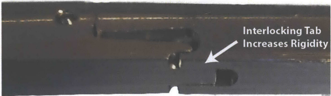
Figure 16: Images showing Hinged Version 3 interlocking tab to prevent “wobble” laterally. Isometric View.
