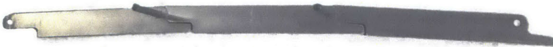
Figure 12: Prototype of Hinged Version 2 produced from 6061 Aluminum using CNC milling processes. Individual segments are pinned together with a carbon steel dowel pin for prototyping purposes.
