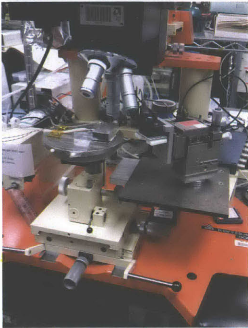
Figure 3-5: Setup used to transfer hBN onto MoS 2 . A stage containing a heating element supports the silicon chip under an optical microscope, while a vacuum keeps the chip stationary. The glass slide holding the transparent polymer stack is mounted upside-down on the transfer arm, which is supported by a magnet that allows coarse adjustments to the hBN position. Micromanipulators on the transfer arm allow fine control of the hBN position and tilt.
