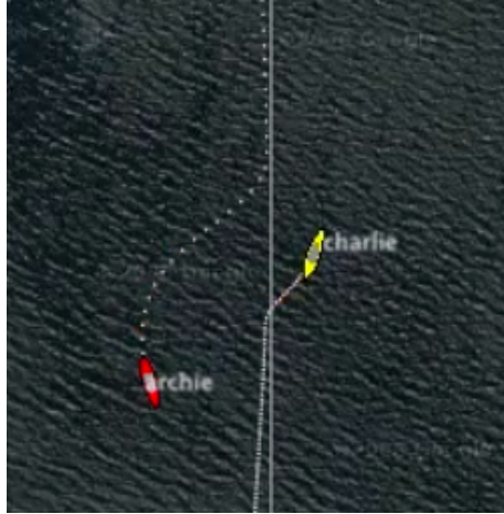
Figure 3-3: Two AMVs approach each other similar to the approaches of Figures 3-1 and 3-2. With COLREGS, the avoidance was much more safe and efficient as seen by reduced track deviation and a lack of either vessel pointing the other after the maneuvers begin. Note the smaller track deviation characteristic of the slower vehicle.
