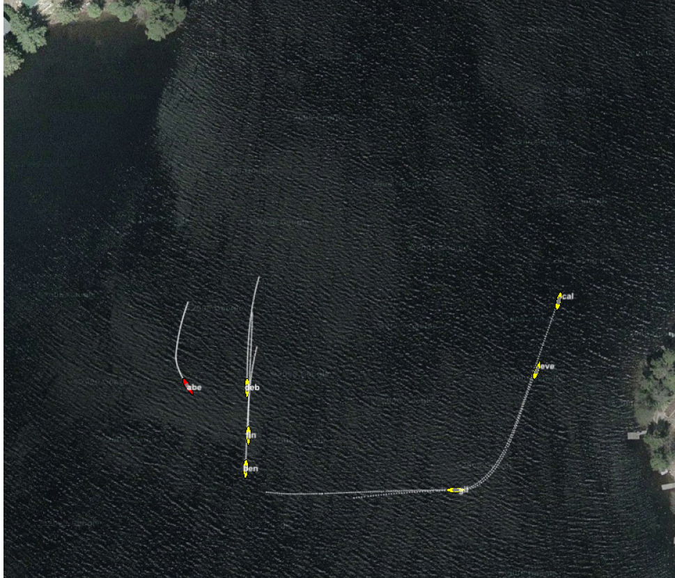
Figure 3-14: The seven vehicle swarm resolved the pattern using collision avoidance with COLREGS until the home plate pattern was achieved with all vehicles.
