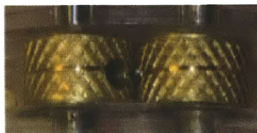
Figure 4-6: Brass knurled drive disks with a center channel to prevent the wire from traveling
