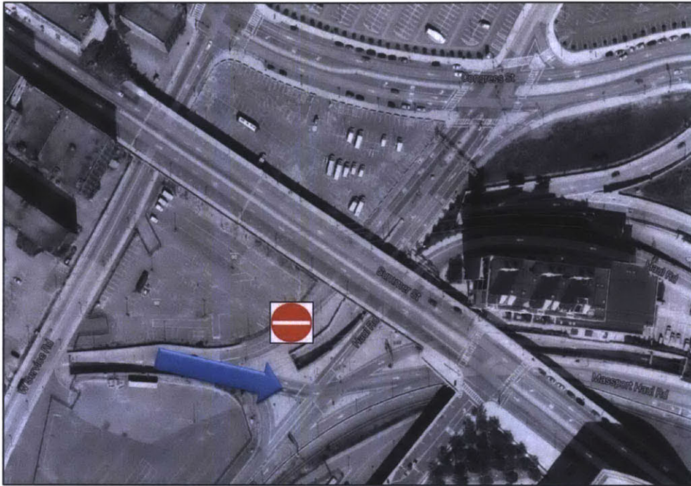
Figure 5-9: Prohibition of the I-90 EB off-ramp
