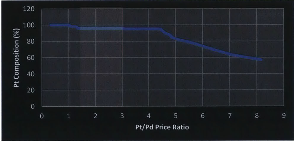
Figure 7: Pt weight fraction as a function of Pt/Pd price ratio for diesel engines.
