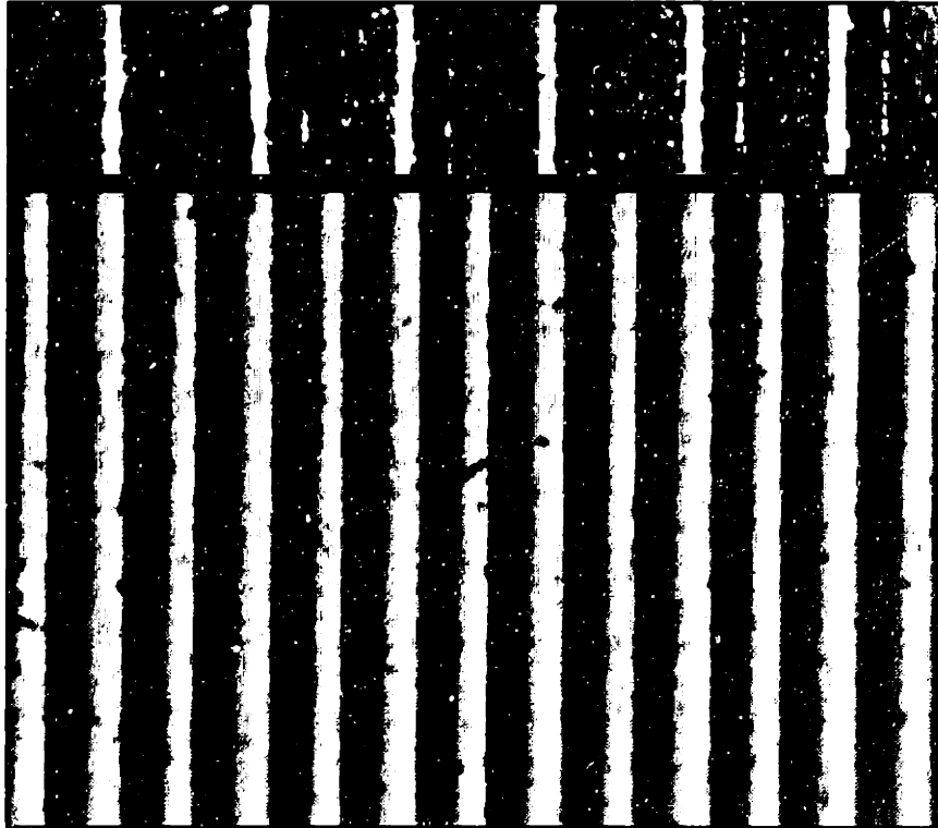
Figure 5.16: Powder bed surface using 35 v/o 1.0 \mu\text{m} alumina slurry, 127 \mu\text{m} nozzle, fast-axis speed of 1.2 m/sec, average flow rate of 1.8 cc/min, and a line spacing of 200 \mu\text{m} (scale divisions are 1/64 inch apart)
