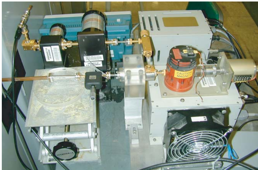
Figure 7-19: The 140 GHz, 200 W EIK driver used in the confocal gyro-TWT experiments. The power supply for the EIK is also shown. A wavemeter and a diode to measure the power and frequency of the BWO is also visible.
