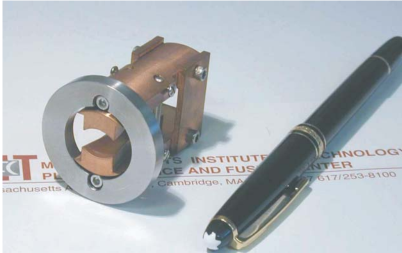
Figure 6-1: The confocal resonator used in the 140 GHz fundamental confocal gyrotron oscillator experiment.
