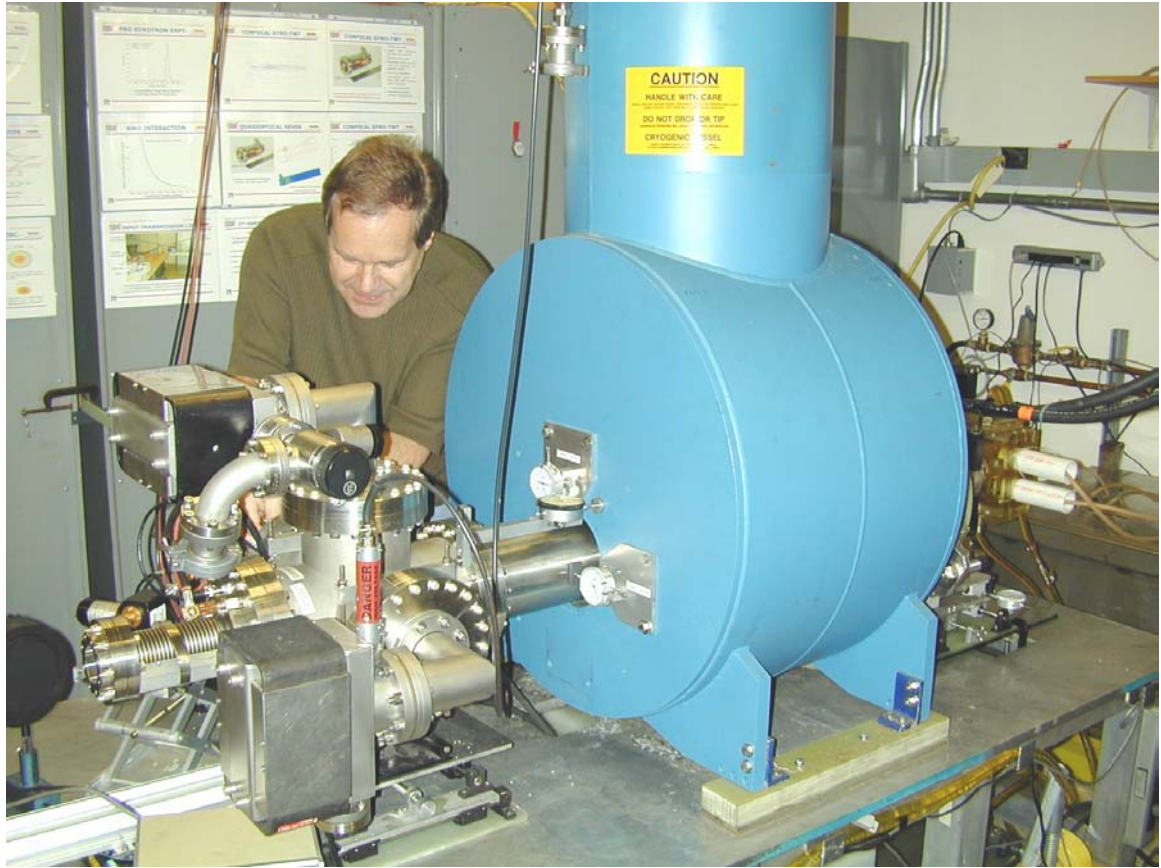
Figure 7-17: The confocal gyro-TWT experiment with Mr. Ivan Mastovsky. The high voltage leads for the electron gun and the high voltage modulator are visible behind the superconducting magnet. The EIK driver (not visible in this picture) is located behind the grey cabinets.
