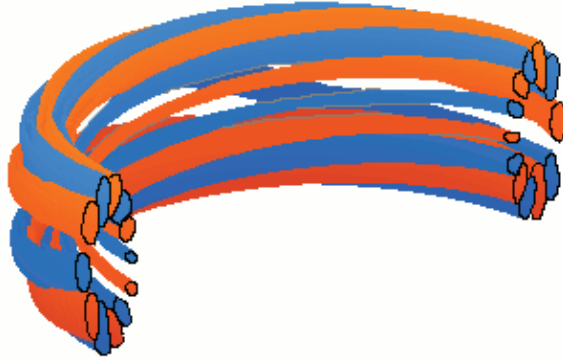
Figure 1-2: Cross-section of the torus illustrating the helical density perturbation (orange is positive and blue is negative) for an Alfvén eigenmode. The structure has a six-fold periodicity in the poloidal plane and a three-fold periodicity in the toroidal plane.
