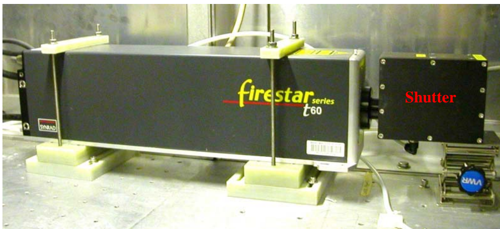
Figure 3-4: Picture of the laser and shutter in the C-Mod PCI system, where the shutter is attached to the laser front.
