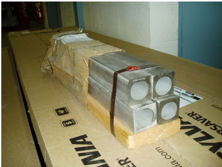
Fig. 1 Four CS1 jacket tubes with 24" each in length
