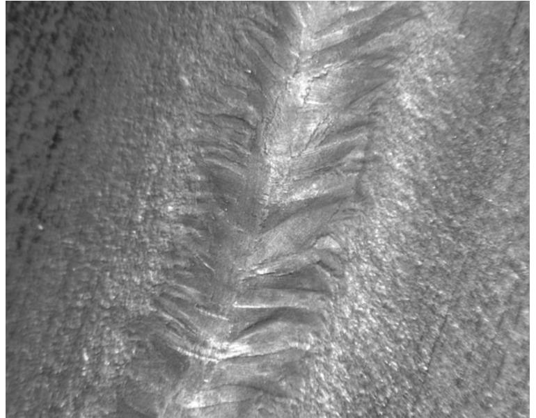
Fig. A1 Typical convex welding with extra deposit in 2 different magnifications (A34)
