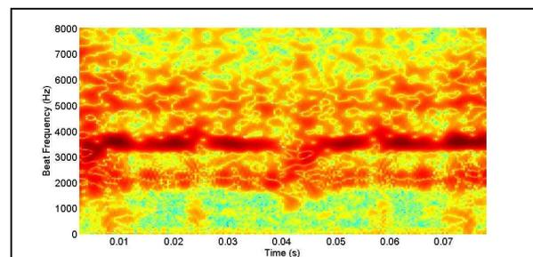
**Figure 5:** Spectrogram of a shot with a reflecting plate 2 meters from the antennas. The plate shows up as a red line (highest intensity) at 3.5 kHz.
