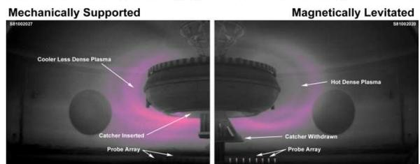
**Figure 1:** Comparison of plasma between mechanically supported and magnetically levitated runs.
