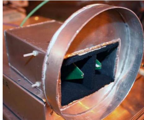
**Figure 4:** Photo of the antenna casing with both log periodic antennas and the Echosorb RF absorbing foam between them.
