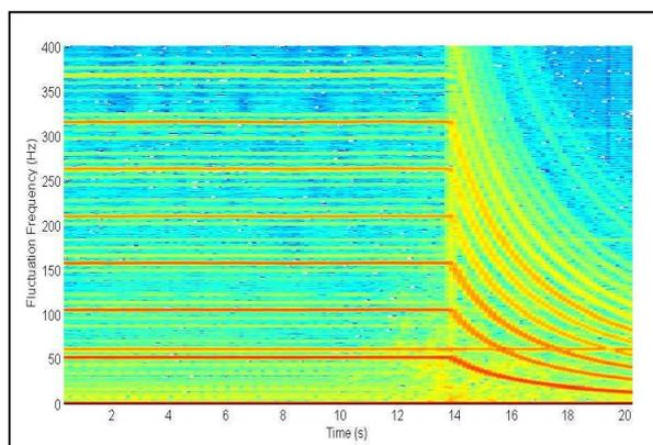
**Figure 8:** Fluctuation frequency versus time throughout at shot. The 3200 rpm (53 Hz) fan is shutoff and slowly decelerates at 14 seconds.
