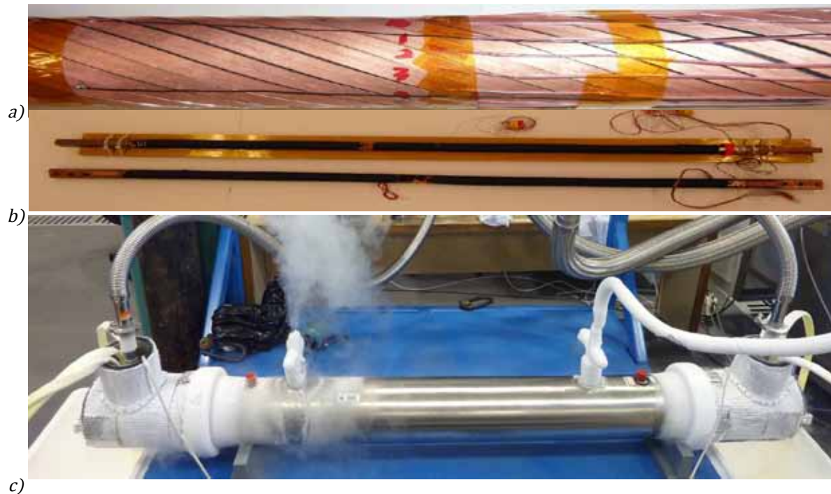
Fig. 6.10: a) Wound cable with voltage taps (left side) and thermo couples (middle). b) Entire cables (two samples) with joints and measuring lines c) Cryostat for test samples (Source: [PKK11])
