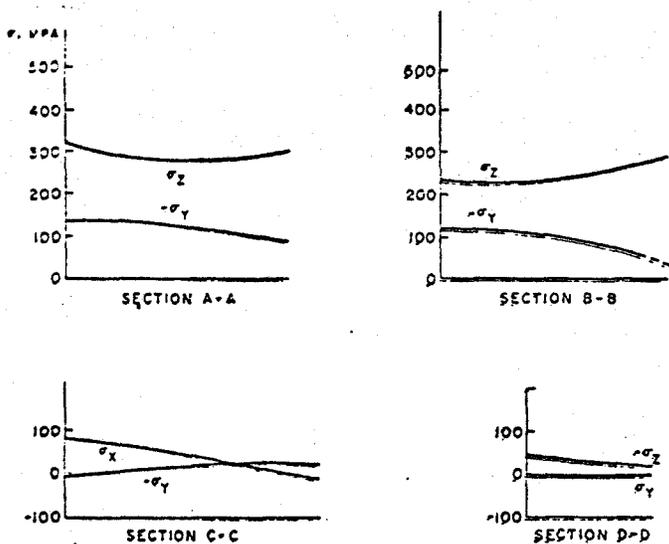
Figure 6 Calculated Copper Stresses Sections indicated in Figure 5.
