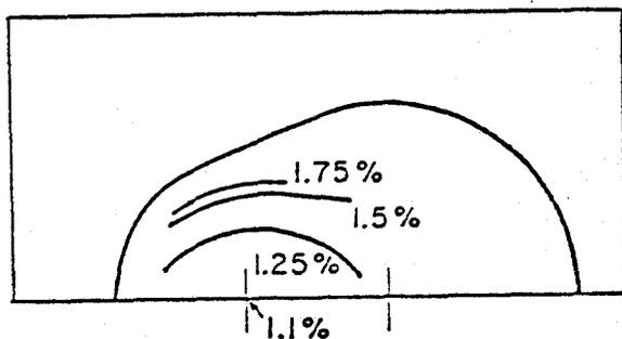
Figure 9 Toroidal Field Ripple due to the Presence of 8 flanges, per Degree of Flange.
