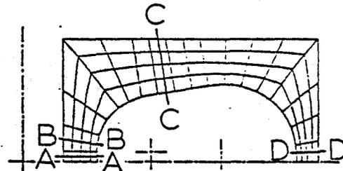
Figure 5 Finite Element Gridwork for Bitter Plate Analysis
