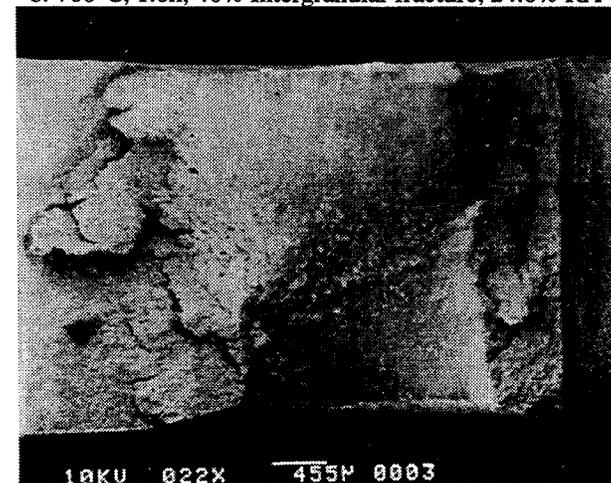
c. 650°C, 114.2h, 47.8% Intergranular fracture, 5.1% RA
