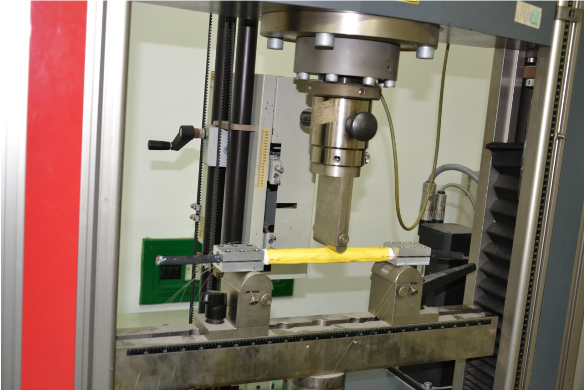
Figure D-3: Three-point-bending test for determining bending stiffness, EI
