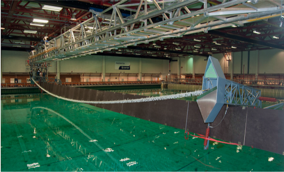
Figure 3-1: The 12mm diameter riser model covered in ribbon fairings. The model is shown mounted on the carriage before it is submerged
