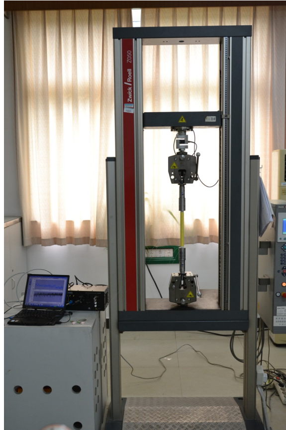
Figure D-1: Tensile test for determining axial stiffness, EA
