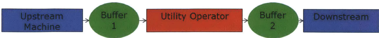
Figure 8.1: Model of production line including the utility operator as a separate machine, a bottleneck between upstream and downstream.
