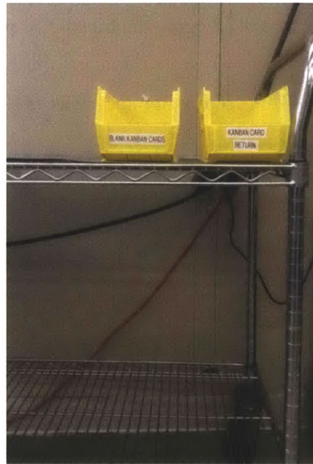
Figure 6.1: Designated bins on supermarket rack for blank and completed Kanban cards.
