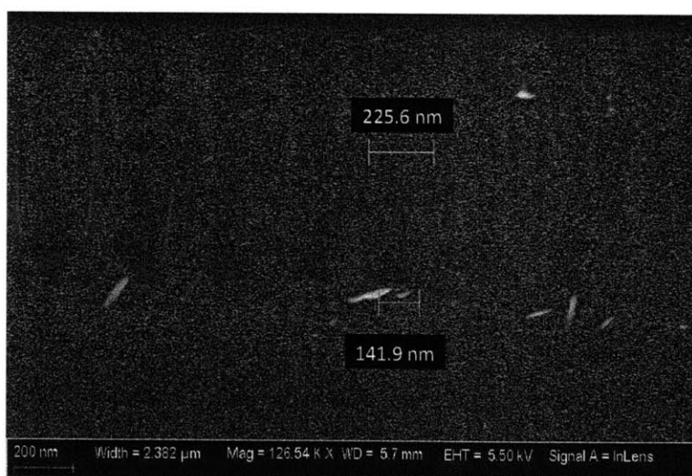
Figure 5-5: SEM image of over-etching from 15 minutes of exposure to hydrofluoric acid, showing widening of the nanohole pores from \sim 150 nm to \sim 225 nm.
