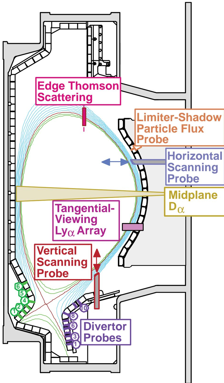
Fig. 1. Cross-section of Alcator C-Mod showing divertor geometry, edge plasma diagnostics and a typical plasma equilibrium used for these studies. Each magnetic flux contour corresponds to a  $\Delta\rho = 2$  mm radial separation at the midplane. In this paper, the separatrix is designated as  $\rho = 0$  and the scrape-off layer as  $\rho > 0$ .
