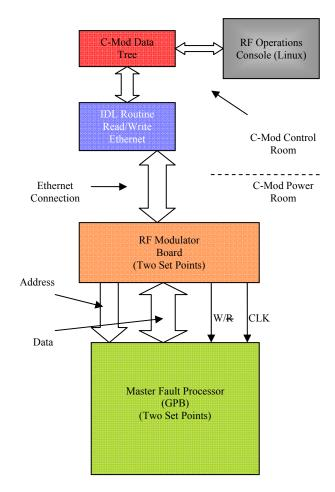
Figure 2. Data Flow Remote Ethernet Connection
