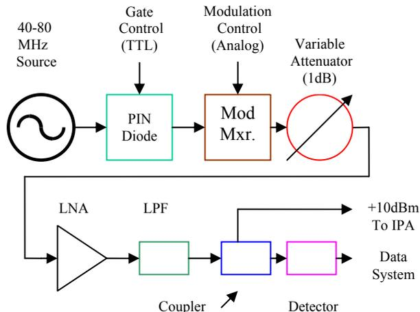
Figure 3. New Low Power Chain For Tunable Transmitters
