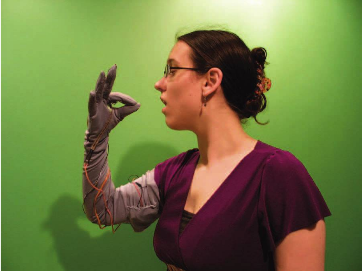
Elena Jessop, the VAMP glove, shown here capturing a note from the singer's voice with a gesture. (© Elena Jessop. Photo: Peter Torpey.)
