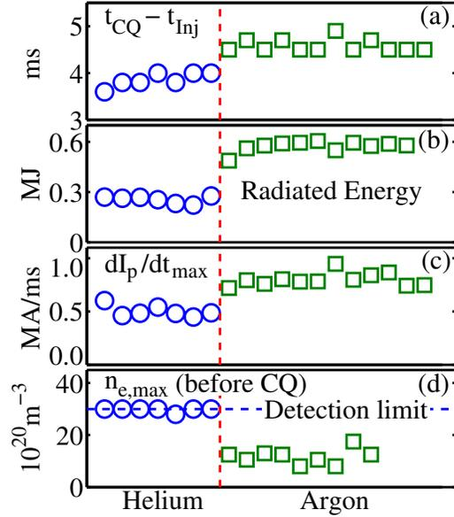
**Figure 1.** Summary of pure He and Ar gas-jet disruption mitigation experiments on Alcator C-Mod [8]. (a) Time delay from start of pressure rise in pipe to beginning of current quench, (b) radiated energy, (c) maximum rate of change of plasma current, (d) electron density  $n_e$  at beginning of current quench. Note  $n_e$  for helium MGI is at detection limits. Neither He nor Ar can fulfill all disruption mitigation requirements.
