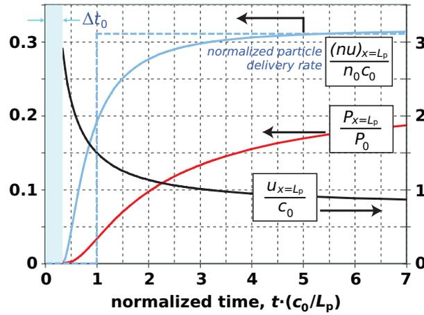
**Figure 2.** Normalized flow rate, pressure, and fluid velocity at the exit of a tube of length  $L_p$  for a reservoir gas of sound speed  $c_0$ .  $\Delta t_0 = L_p/3c_0$  is the time at which the gas first arrives at the pipe exit.
