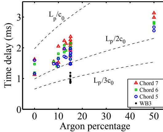
**Figure 6.** The time of the collapse of the edge soft X-ray signals correlates with the time of the arrival of the gas to the plasma for argon/helium mixtures. Blue circles: chord 5 ( $r/a = 0.96$ ), green squares: chord 6 ( $r/a = 0.91$ ), red triangles: chord 7 ( $r/a = 0.87$ ). A fast photodiode pointing directly at the gas jet [16] indicates the arrival of the gas at the plasma. Dashed lines indicate the modelled gas arrival time  $L_p/3c_0$  and the sonic transit time  $L_p/c_0$ .
