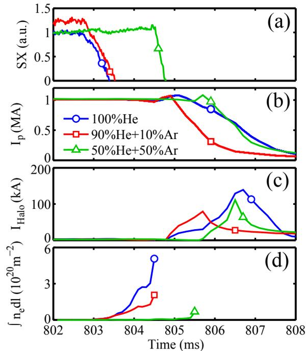
**Figure 4.** Waveforms of (a) edge soft X-ray signal, (b) plasma current, (c) halo current, (d) chord-integrated electron density for 3 disruption mitigations using pure helium (blue circle), a mixture of 90% He + 10% Ar (red square), and a mix of 50% He + 50% Ar (green triangle).
