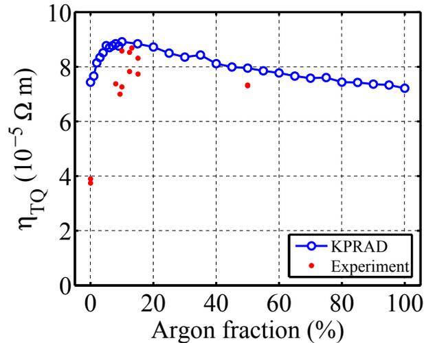
**Figure 10.** Observed (from current decay  $L/R$  timescale) and calculated (KPRAD) resistivity of the plasma immediately after the thermal quench, for helium-argon mixtures. Using a mixture of approximately 15–20% Ar forces the plasma to a highly resistive phase.
