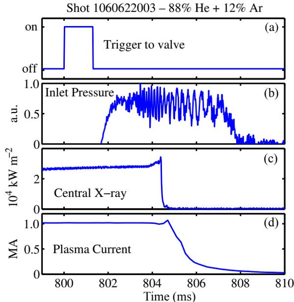
**Figure 3.** Waveforms for C-Mod shot 1060622003, a typical disruption mitigation experiment using a mixture of 88% He + 12% Ar. (a) Current applied to the valve, (b) pressure at the valve outlet, (c) central soft X-ray intensity, (d) plasma current.
