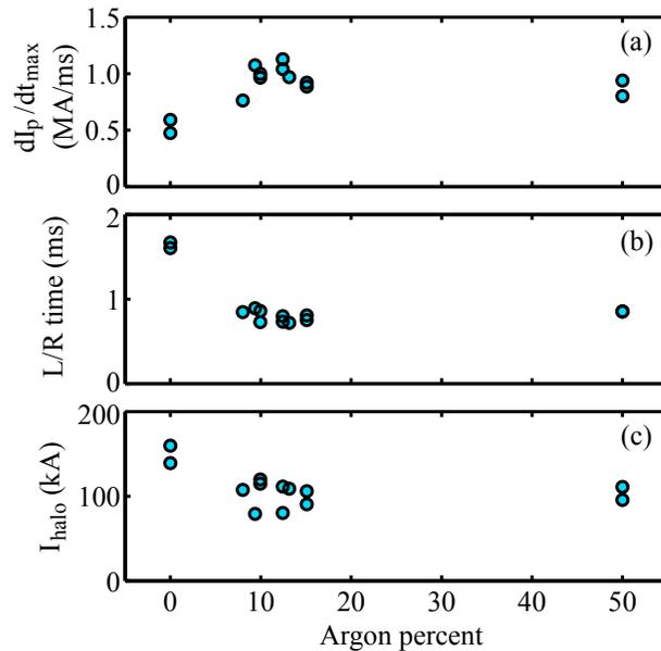
**Figure 8.** (a) Helium/argon mixtures with low argon fractions produce the maximum current quench rates. (b) The L/R current-decay timescale in all Ar/He mixtures is lower than that in pure helium, and consequently the peak halo current (c) is lower using gas mixtures.
