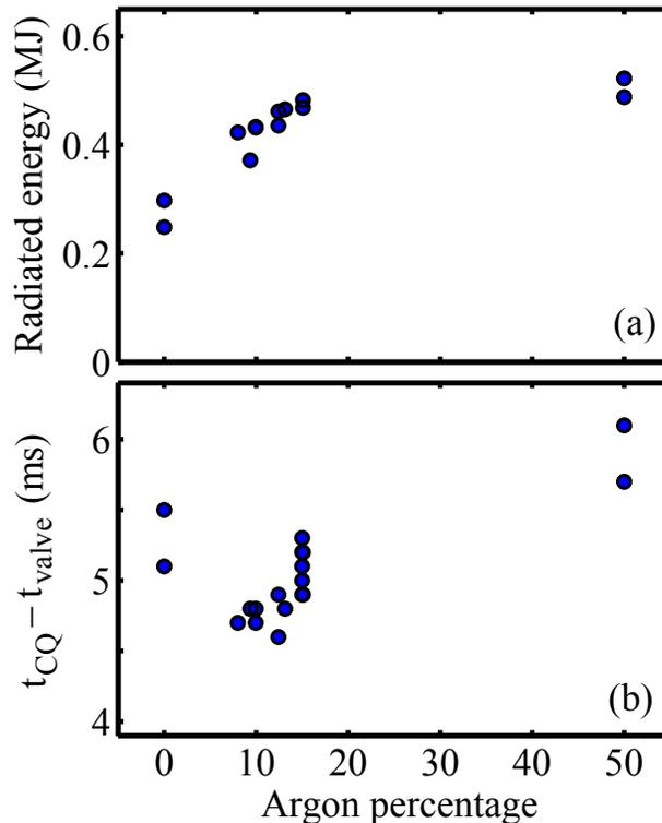
**Figure 7.** Radiated energy during thermal quench and delay time from signal sent to valve, to start of current quench, for mixtures of argon/helium. (a) For argon fractions less than approximately 20%, the radiated energy during the thermal quench increases with the argon fraction. (b) The delay to the start of the current quench is a minimum for argon fractions of approximately 10–15%.
