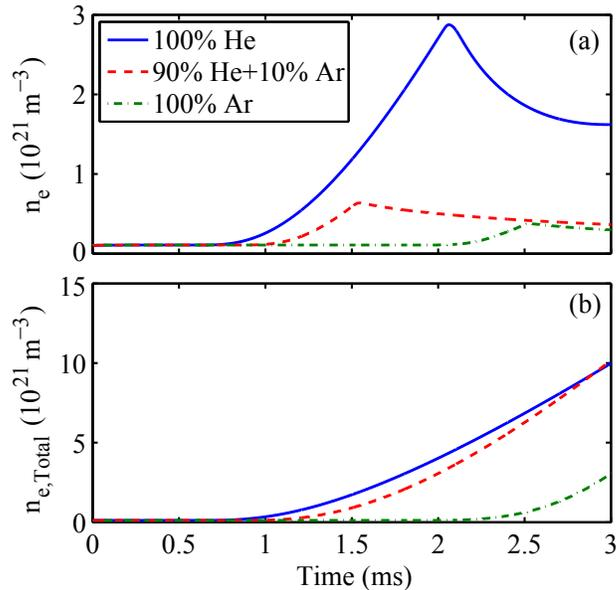
**Figure 9.** (a) The simulated free electron density agrees well with the experimental results (see figure 4d). In the case of helium-argon gas mixtures, the contribution of the argon to the density increment is  $\sim 20\%$ . (b) Similar total (free + bound) electron density is obtained using pure He and 90% He + 10% Ar.
