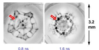
FIG. 4 (Color online) Proton fluence images of capsule implosions driven by gas-filled hohlraums. The open arrows point to interfaces between Au wall blow-off and gas plasma. A relatively smooth interface appears between the expanding wall blow-off and the ionized fill gas at time 0.8 ns, while chaotic spatial structure and interface interpenetration are evident at time 1.6 ns. The fluence surplus inside the imploding capsule (0.8 ns) resulted from self-generated radial *E* fields [22,23].
