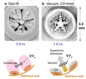
FIG. 3. (Color) The proton fluence distributions are showing surplus in the regions between the pairs of expanding plasma plumes in a gasfilled, Au hohlraum (a) but showing deficit in a CH-lined, vacuum Au hohlraum (b), indicating opposing directions of the self-generated electric fields as illustrated schematically by the corresponding cartoons.
