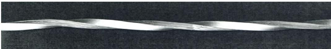
Fig. 3. Schematic illustrations of twisted stacked-HTS tape conductor.
