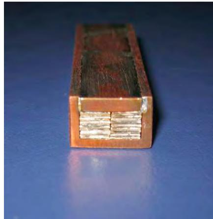
Figure 4. Untwisted cable developed at NIFS.
