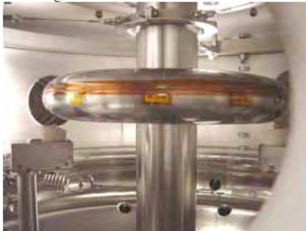
Fig. 17. Levitated coil in mini-RT experiment at the University of Tokyo.
