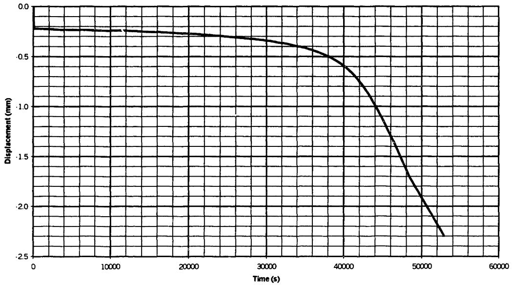
Displacement vs. Time Si 1000 \mu m, 9x45+mm, 600°C 45.5N
