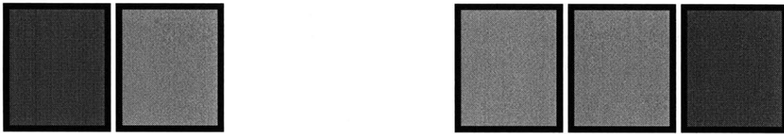
Figure 2-14: A visual tag representing the value ten. Squares at either end are red while the inner squares representing the bits are green.
