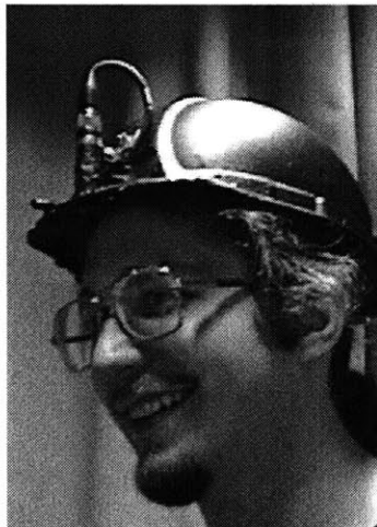
Figure 2-11: A hard hat adapted for mounting downward- and forward-facing cameras.
