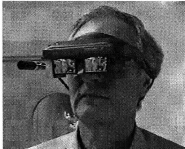
Figure 2-8: A head-mounted camera and a head-up display connected wirelessly to a SGI can simulate a powerful wearable computer for augmented reality.
