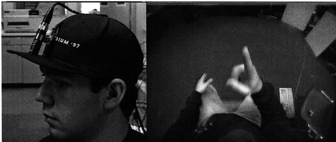
Figure 2-10: The hat-mounted camera, pointed downward to the hands, and the corresponding view.
