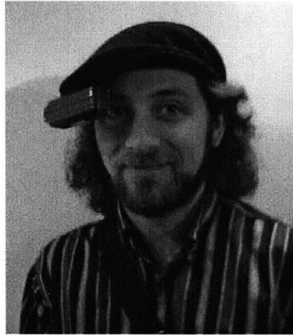
Figure 2-1: A Private Eye mounted in the brim of a hat.
