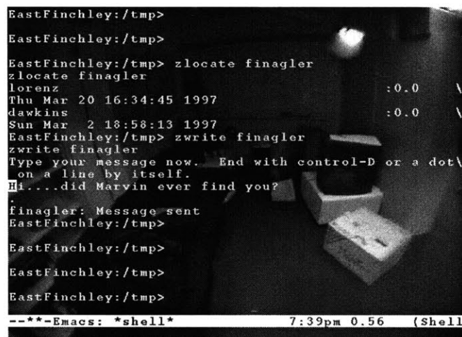
Figure 2-4: In fact, the user's brain fuses the image from the monocular display with the image of the world.
