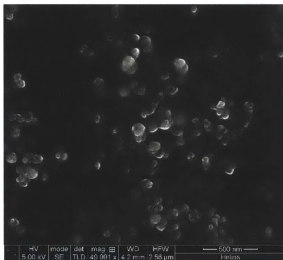
Figure 6-2 SEM/FIB images at different magnifications of surface coatings obtained from nanofluid boiling.
