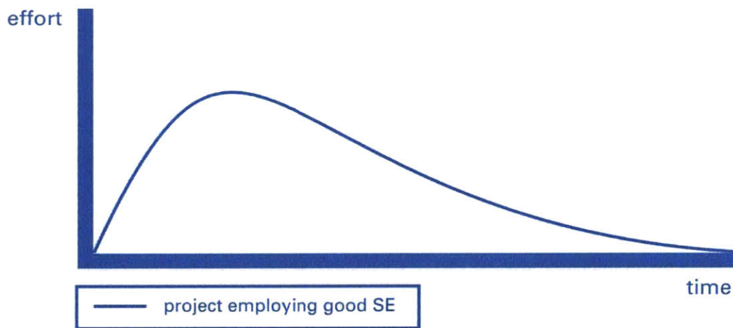
Figure 31. Standard Rayleigh curve distribution of effort (manpower hours) versus time for project development. 157 If plotted from SCR, this curve is the approximate derivative of the expenditure curve depicted in Figure 30.
