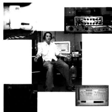
Figure 8: Photograph of Skinscape system. (a) V1220 transducer located on wrist; (b) Velcro adjustable elastic band; (c) Interactor cushion amplifier unit; (d) 12-channel V1220 amplifier unit; (e) Digi001 hardware interface; (f) ATX-M3H headphones; (g) Macintosh G4; (h) screenshot of ProTools LE audio editing environment. (From (Gunther, 2001))
