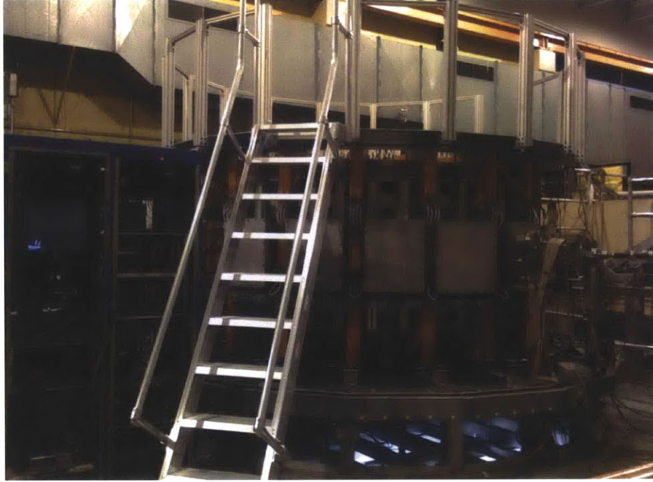
Figure 2-1: A photograph of VTF. Note the horizontal ports, stairs to the top of the machine where half of the vertical ports are located (the other half are on the bottom of the machine), orange toroidal magnetic field coils, and some of the computers and electronics for data acquisition.
