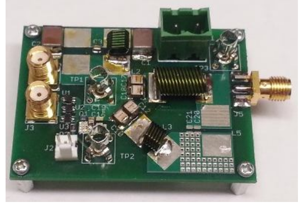
Fig. 11. Photograph of the traditional \Phi_2 inverter designed according to [27] (see Fig. 13a). PCB size is 42 mm x 57mm. The transformed version of the \Phi_2 inverter (Fig. 13d) has an identical PCB layout, although it is populated with different components.
