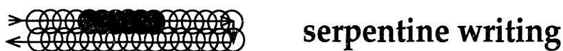
Figure 2: Representation of a coordinated maskless writing strategy in ZPAL. The stage scans while the multiplexing unit selects which zone plates shall expose pixels.
