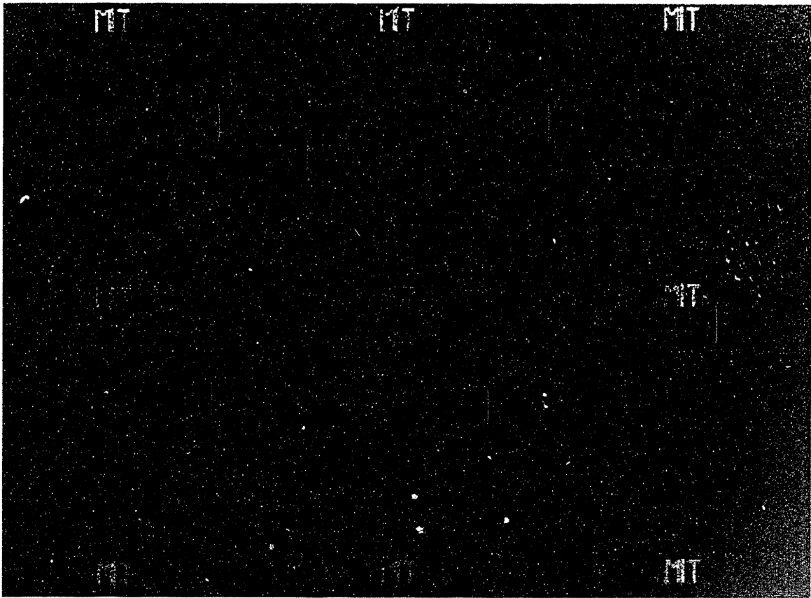
Figure 17: Scanning electron micrograph of nine arbitrary patterns written in parallel in PMMA and developed.
