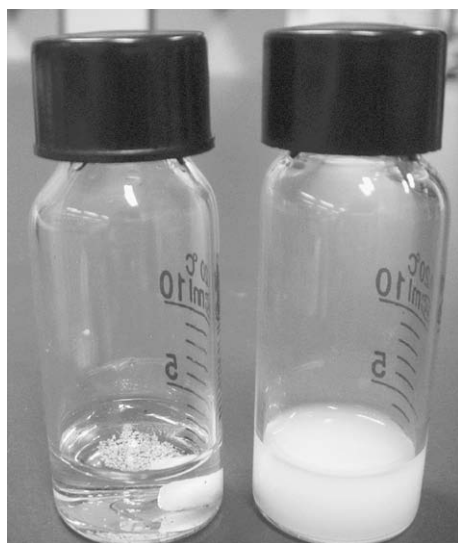
Fig. 2. Pyrene ( [\text{Py}] = 4.45 \times 10^{-3} \text{ M} ) in deionized water (left), and the peptide–pyrene solution ( [\text{Py}] = 4.45 \times 10^{-3} \text{ M} , [\text{Peptide}] = 3.79 \times 10^{-4} \text{ M} ) (right) after stirring for about 2 h.
