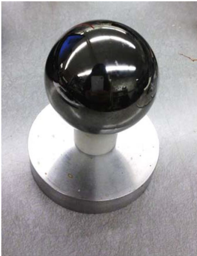
Figure 2-6: Rotor sphere for magnetic suspended reaction sphere prototyping.
