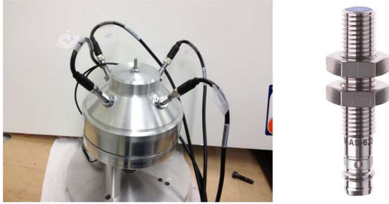
Figure 2-4: Inductive sensors for sphere position sensing and their arrangement as 4 symmetrically locate probes.
