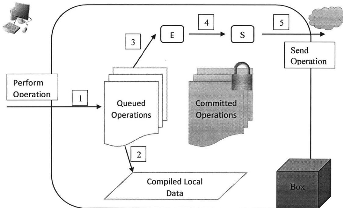
FIGURE 3 THE PROCESS AN OPERATION GOES THROUGH FROM WHEN THE CLIENT PERFORMS IT UNTIL IT REACHES THE CLOUD. NOTE THAT E=ENCRYPT, AND S=SIGN.
