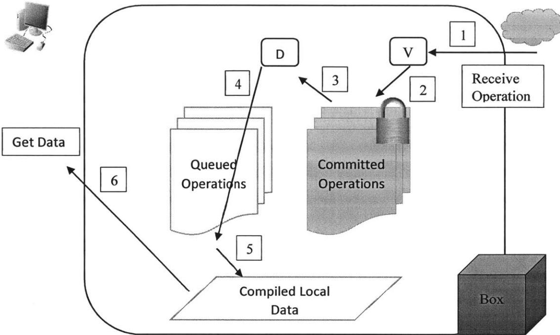
FIGURE 2 THE PROCESS AN OPERATION GOES THROUGH FROM WHEN THE CLIENT'S BOX RECEIVES AN OPERATION UNTIL IT IS READ BY THE USER. NOTE THAT D=DECRYPT, AND V=VERIFY.
