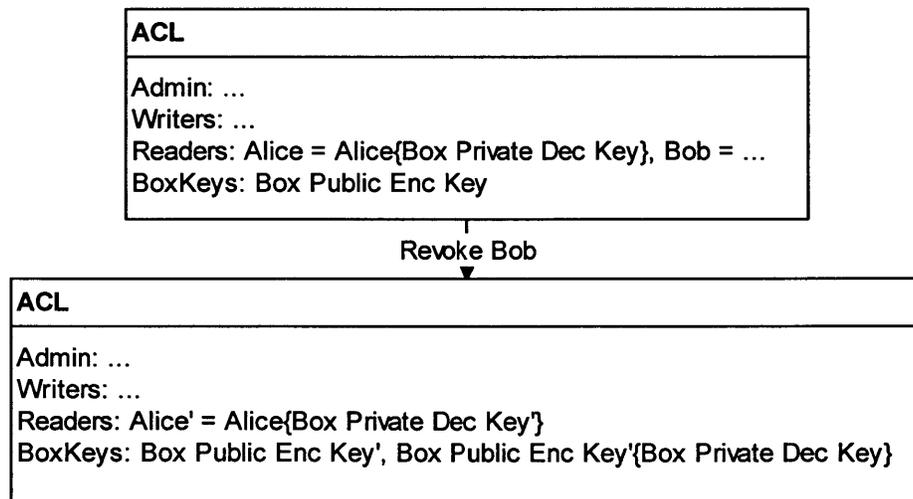
**FIGURE 7 THE ACL OF AN OBJECT BEFORE AND AFTER BOB’S READ ACCESS TO THE OBJECT IS REVOKED. THE NOTATION  $A\{B\}$  MEANS THAT THE KEY B IS ENCRYPTED UNDER THE KEY A. ADDITIONALLY, THE NOTATION  $X'$  MEANS THAT X HAS CHANGED. FINALLY THE NOTATION  $ALICE' = ALICE\{BOX PRIVATE DEC KEY'\}$  MEANS THAT ALICE’S NEW READ PERMISSION IS DEFINED BY HER PUBLIC KEY WRAPPING THE NEW BOX PRIVATE KEY.**
