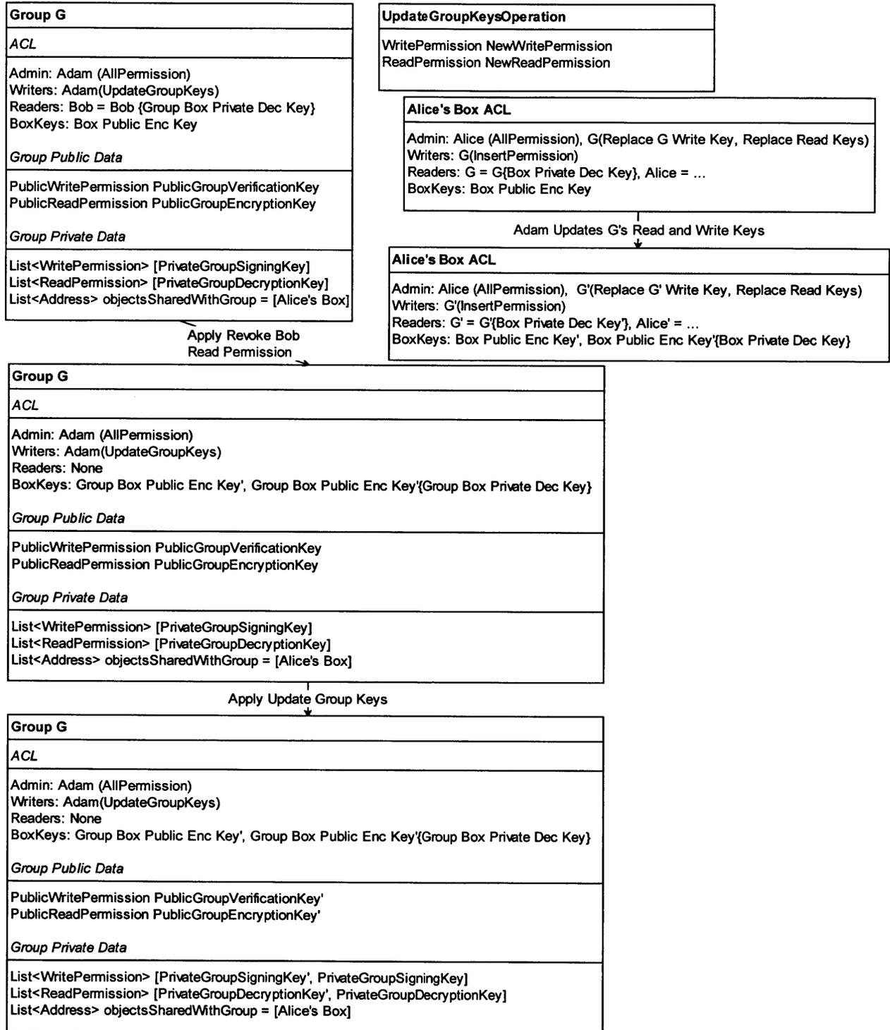
FIGURE 10 THE MODIFICATION OF GROUP G AND ALICE'S BOX WHICH IS SHARED WITH G, AS BOB IS REMOVED FROM G.
