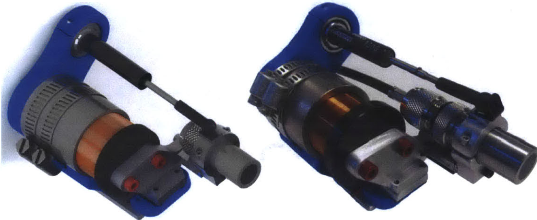
Figure 7-7: Solid model rendering (left) and photo (right) of the dynamic imaging probe, Version 2, designed to accommodate a single-element Olympus ultrasonic transducer, and to address the limitations of Version 1.
