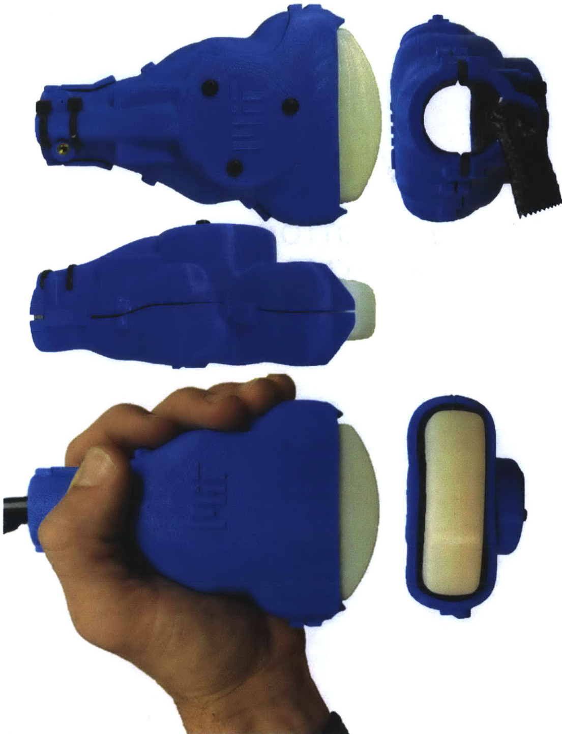
Figure 3-5: Front, side, and back views of the six-axis force/torque-measuring ultrasound probe. Depicted with a 3D-printed ultrasound probe mock-up.
