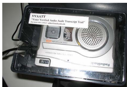
Figure 8: VVAATT audio recorder in protective box.
