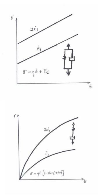
Which of these rheological bodies shows recovery from deformation when the load has been removed? 5. The Boltzmann equation (integral representation of the constitutive equation)
