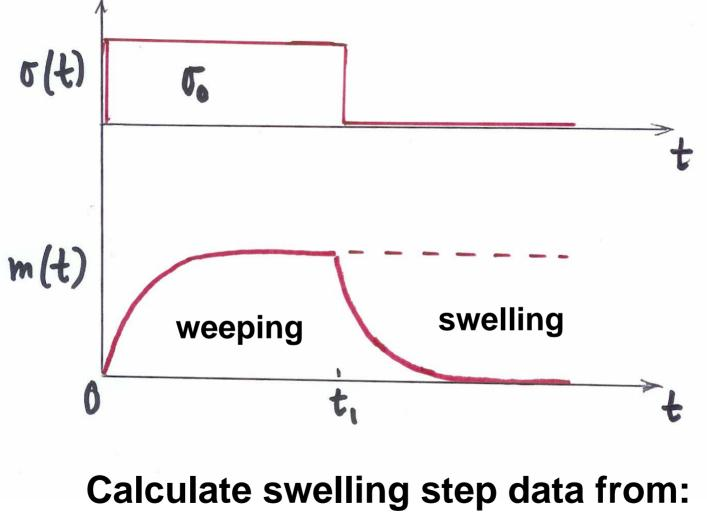
Calculate swelling step data from:  $m(t) = \sigma_o W - \sigma_o W(t - t_1)$
