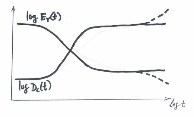
Data show the evolution of  $E_r(t)$  and  $D_c(t)$  for an amorphous synthetic polymer over about 20 decades of logarithmic time. These "master curves" can be obtained in a morning using time-temperature superposition.
