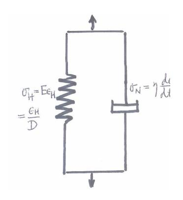
Kelvin-Voigt model. **Derivation of** equation of motion (constitutive equation for creep at constant stress)
