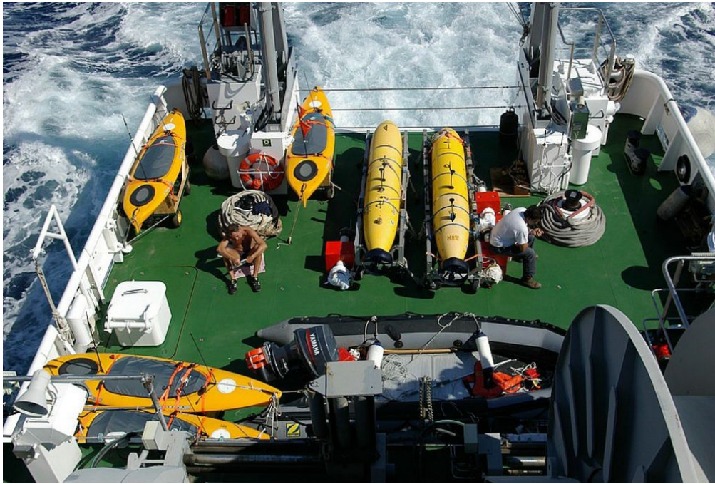
FIGURE 7 Autonomous underwater vehicles (Odyssey II) and surface vehicles (kayak hulls) are essential to every oceanographic cruise and become increasingly important to naval operations ( photo courtesy of John Leonard ).
