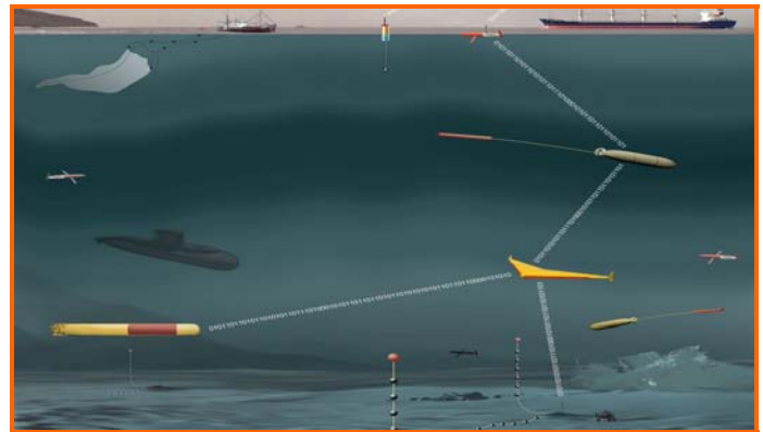
FIGURE 8 Multiple coordinating AUVs, gliders and surface craft, guided by Global Positioning System or submerged vehicles will offer a unique capability to map and explore the ocean on a scale that was unimaginable a decade ago.
