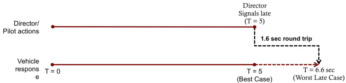
Figure 5-7: Diagram of worst-case scenario for RT latency effects for a five-second task. Upper timeline shows Director and Pilot actions, bottom timeline shows vehicle response to Pilot commands. If Director provides command late (at the 5 second mark) and the Pilot does not preemptively stop the aircraft, the round-trip 1.6 second latency in communicating the “STOP” command to the vehicle, the pilot issuing the command, and the command being executed causes the vehicle to stop late. The task completes at 6.6 seconds.
