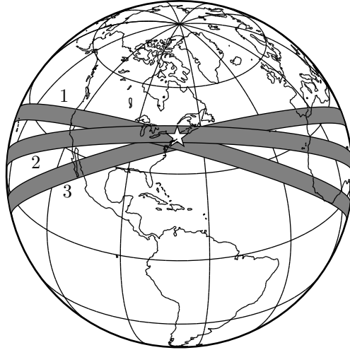
Figure 6-41: The repeat coverage orbit, where inclination is matched to the target latitude, can provide coverage on successive orbits
