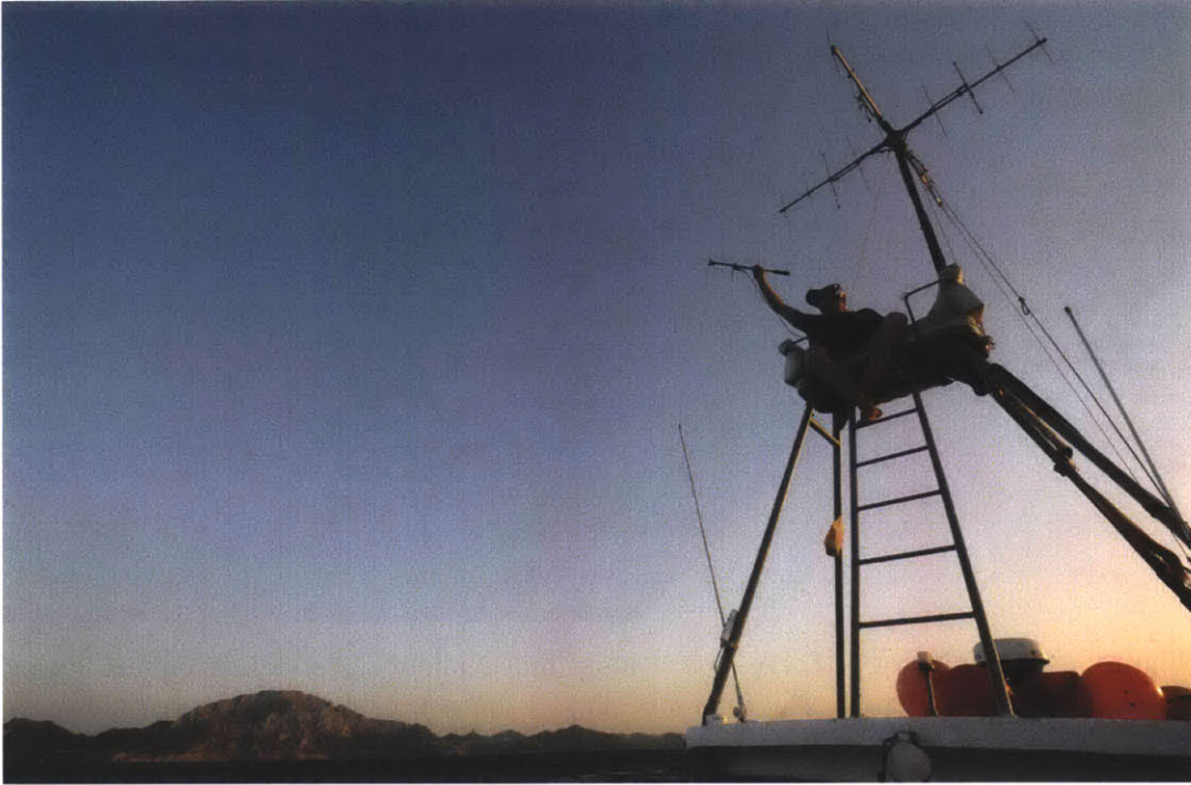
Figure 4-3: Radio-tracking a DTAG deployed on a pilot whale using a hand-held VHF antenna. Photo credit: Frants Jensen
