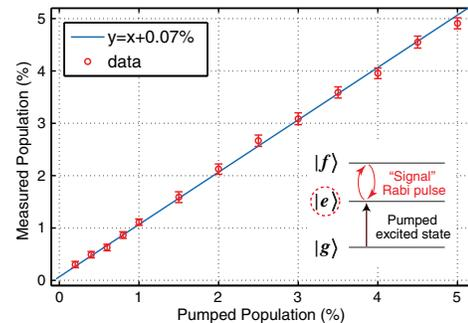
FIG. 2 (color online). Calibration measurement of excited state population (percent), pumped using a small fraction of a  $\pi^{g \rightarrow e}$  pulse. The data can be fit to a linear  $y = x + b$  function, where  $b = 0.067\%$ , with 95% confidence bounds of (0.025%, 0.011%).
