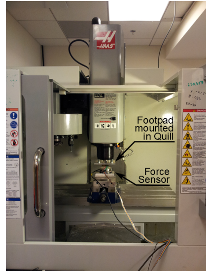
(a) CNC milling machine with the footpad and F/T sensor mounted within.
