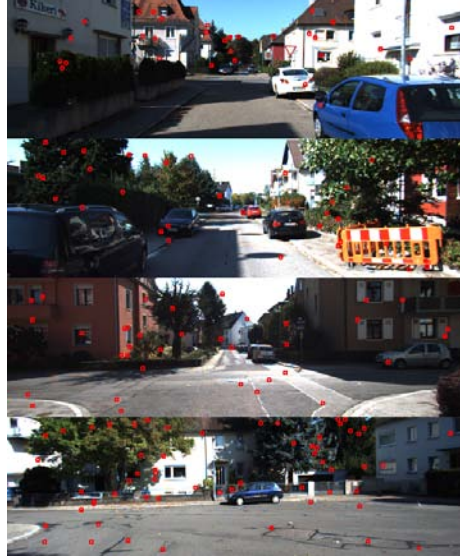
Figure 23: Typical camera images from the test KITTI dataset. Features tracked by the visual odometry system are indicated in red.
