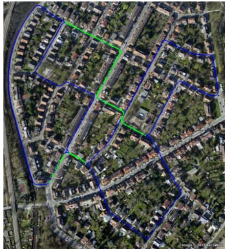
Figure 24: Ground truth trajectory (blue) with areas of identified feature correspondences (loop closures) identified (green).
