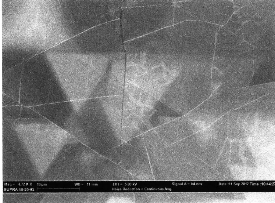
Figure 2-13: Scanning Electron Microscopy of Large Area hexagonal boron nitride synthesized on Iron foils from Dr. Ki Kang Kim.
